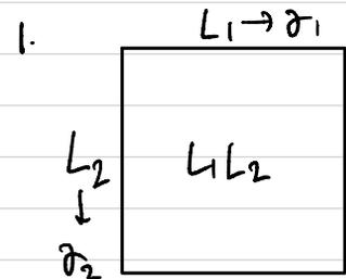
$$\begin{aligned}\Delta G &= \int \sigma dl \\ &= 2 \times \int_0^{L_1} \sigma_1 dl + 2 \times \int_0^{L_2} \sigma_2 dl \\ &= 2\sigma_1 L_1 + 2\sigma_2 L_2\end{aligned}$$
