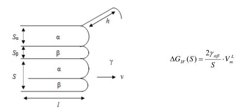
where  $\gamma_{\alpha\beta}$  is the  $\alpha/\beta$  interfacial energy and  $V_m^L$  is the molar volume of the lamellar structure.
