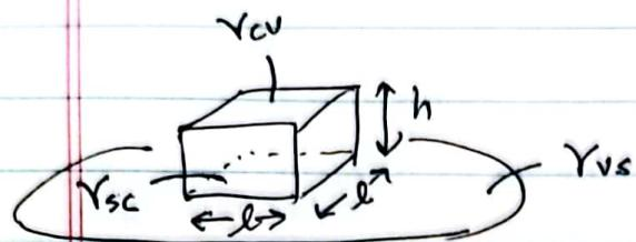
$$\begin{aligned}\Delta G &= -l^2 h \Delta G_v + l^2 Y_{cv} + 4lh Y_{cv} + l^2 Y_{sc} - l^2 Y_{vs} \\ &= -l^2 h \Delta G_v + l^2 \Delta Y + 4lh Y_{cv} \quad (\Delta Y = Y_{cv} + Y_{sc} - Y_{vs})\end{aligned}$$
