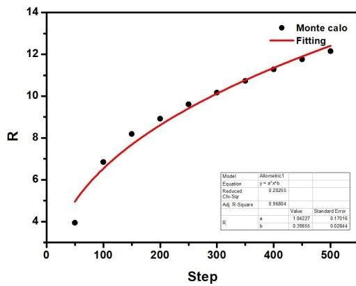
(a)  $R = k t^n$ . simulation result.  $y = a x^b \rightarrow a = 1.042$
